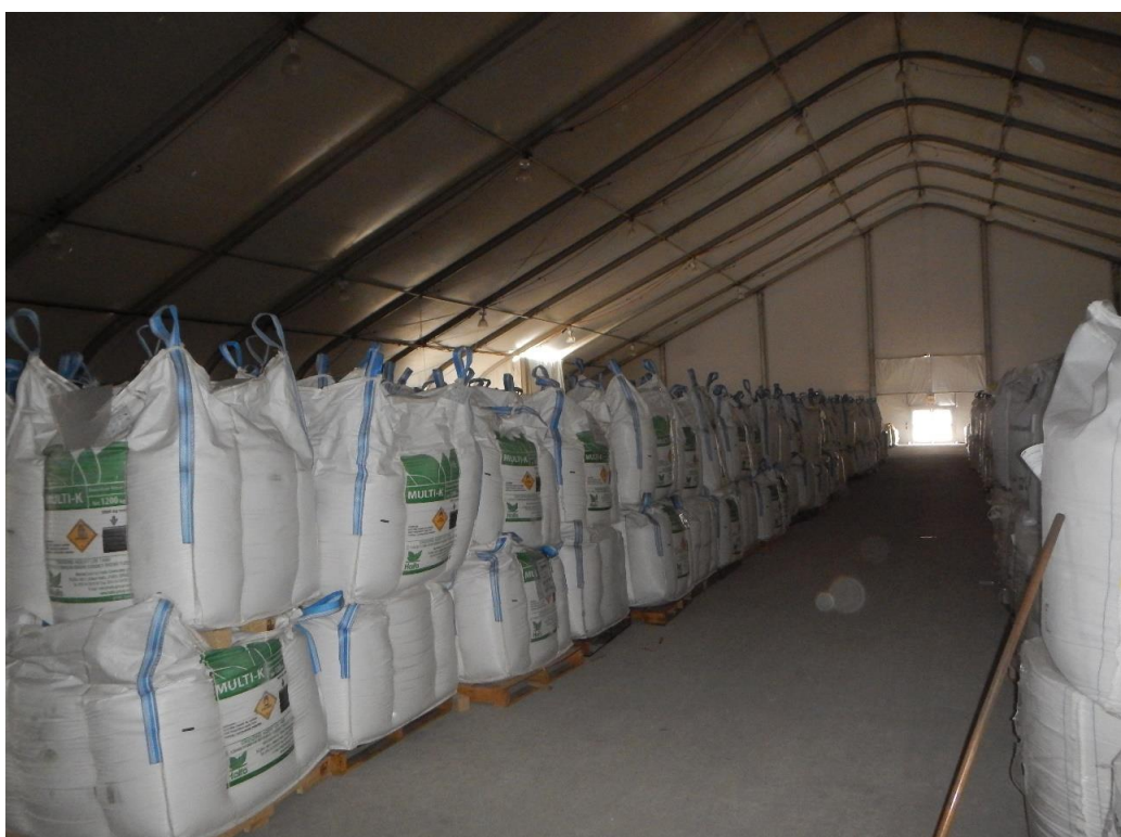
Figure 8 Intermediate storage of nitrate salts before mixing and processing at a melting station [3]
